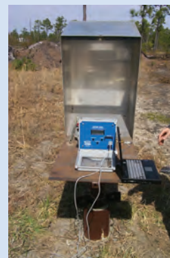
Satron 8400 recorder installation with laptop for data download. (Photograph by Bill Cunningham, USGS)
