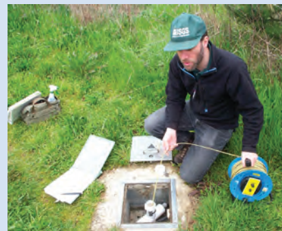
Field measurement with electric tape. (Photograph by Bill Cunningham, USGS)
