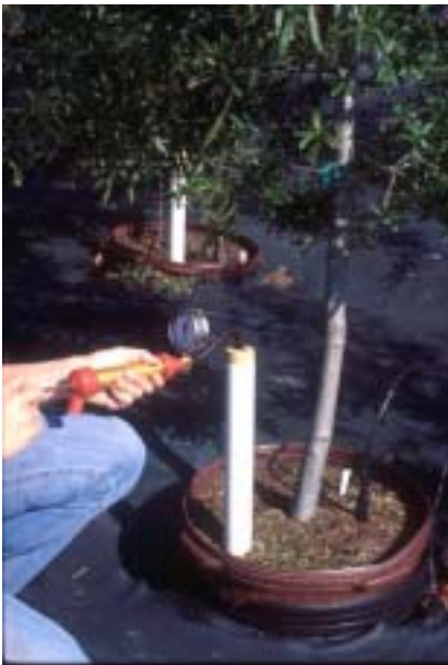
Fig. 2. Vacuum being drawn on a suction cup lysimeter in a 15 gallon in-ground container.
