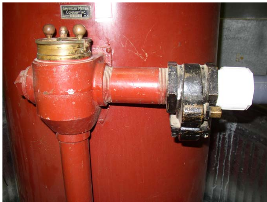
Valves on Bell Prover. Open relief valve on left to raise bell. Use wrench on bypass valve on right.
