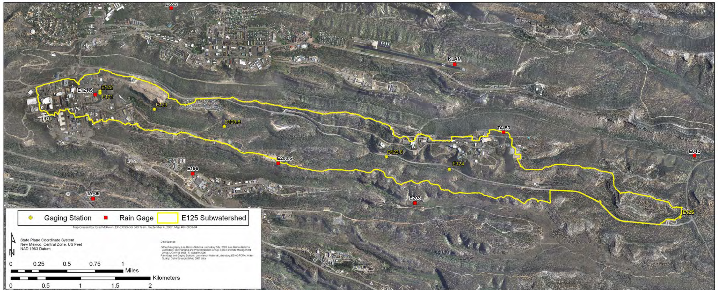
Figure B-1 Orthophotograph of Sandia Canyon on Laboratory land showing locations of gaging stations and precipitation stations used in this appendix and the extent of the drainage basin upcanyon from gaging station E125
