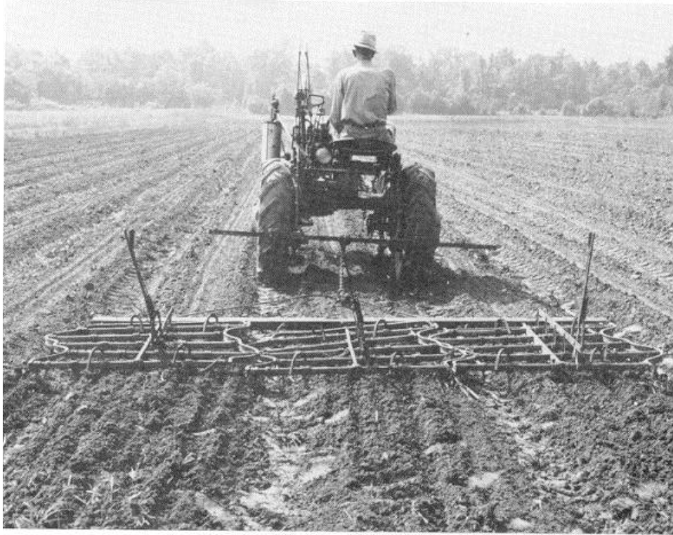
FIGURE 15.—Three-section spike-tooth harrow preparing the seedbed for sorgo.
