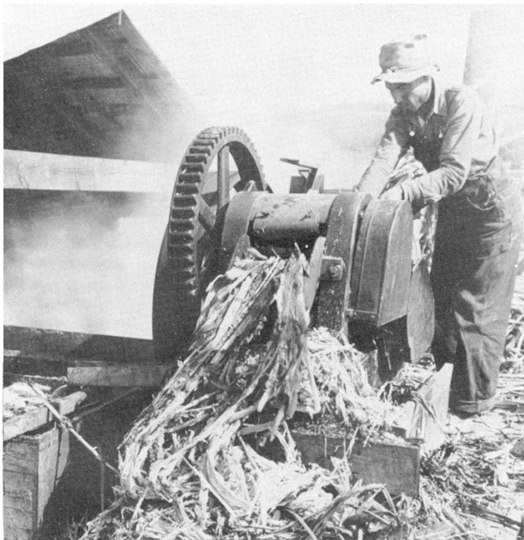
FIGURE 24.—Grinding sorgo at a sirup mill in Coosa County, Ala. Note the juice coming out of trough.
