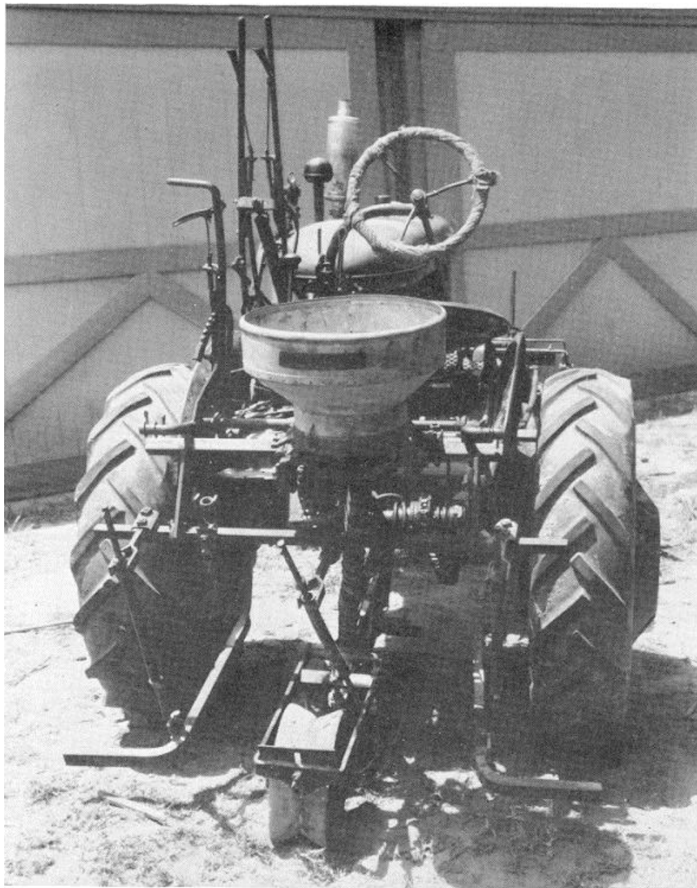
FIGURE 18.—A tractor-operated planter equipped with a knife-type opener.
