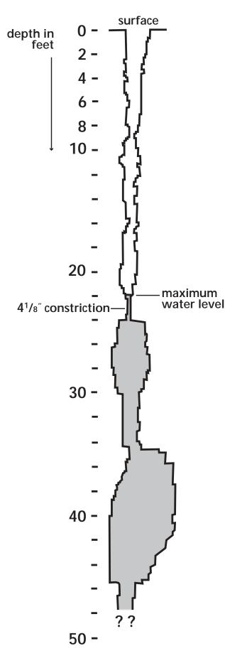
Geyser tubes or "plumbing systems" are not uniform in shape. They are usually crooked or constricted in many places. Measurements of Old Faithful's conduit reveal a constriction at about 22 feet (6.7 m).
