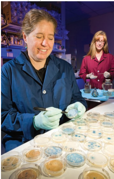
Microbiologist Jean McLain (left) examines bacterial colonies in petri dishes as technician Sharette Evans prepares more soil and water samples for analysis. Dark-blue colonies, presumptive for E. coli , will be isolated and tested for false positives.
