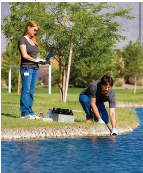
Technicians Allan Knopf and Sharette Evans collect water samples from a pond that supplies irrigation water to Pacana Park in Maricopa, Arizona. In the laboratory, the pond-water samples are filtered to isolate microbes. DNA extracted from the filters is then screened for the presence of human-specific Bacteroides molecular markers.
