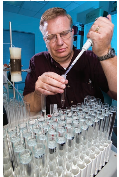
Soil scientist Clinton Williams prepares for analysis of water samples from a municipal park being irrigated with reclaimed water. The test will determine the fate and transport of the human drug carbamazepine.
