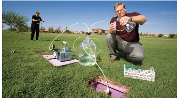
In Pacana Park, Clinton Williams draws water samples from large lysimeters installed under the turf while Jean McLain collects soil samples to assess downward bacterial transport from the surface.
