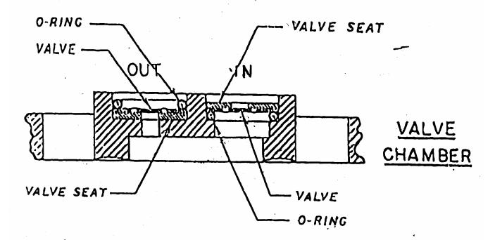
NOTE: ASSEMBLE VALVE COMPONENTS IN ORDER SHOWN.
