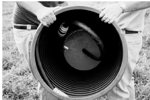
Figure 11. Inside of Sling Pump
