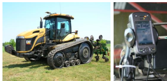
Figure 2. Tractor equipped with RTK GPS receiver and internet accessible cellular phone which receives real-time GPS correction signal from a CORS site in Lawrence County, Alabama.
