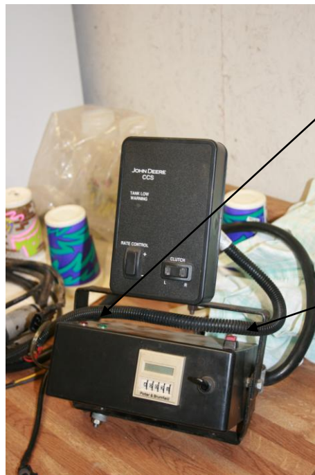
This is a photo of the counter that indicates when the tramlines should be planted. It is set to activate the linear actuator on the second of every three passes.
