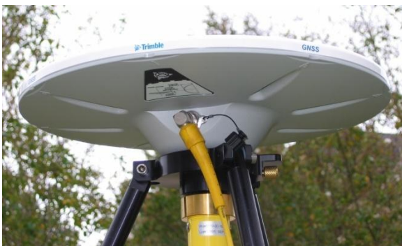
Figure 1. Example of a Trimble® GNSS-compatible antenna. Note the “GNSS” label on the rim. Most compatible antennas/receivers will have this label.
