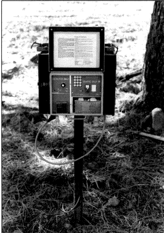
Figure 23-Traffic counters record numbers of vehicles in 1 5-minute blocks and operate continuously from May through December.
