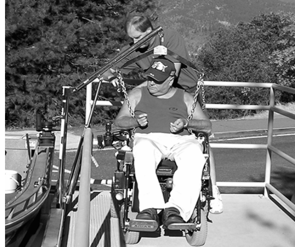
Accessible loading platform and slip for a patient lift at Centimudi public boat ramp at Shasta Lake.
