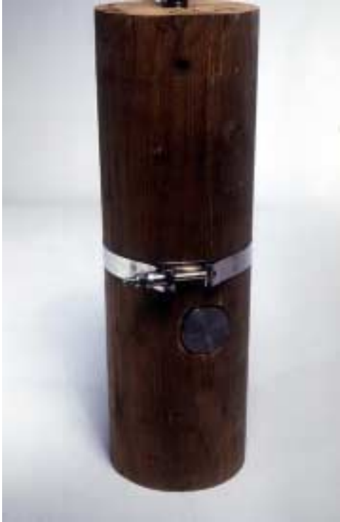
Figure 1. Dowel-nut connection detail
