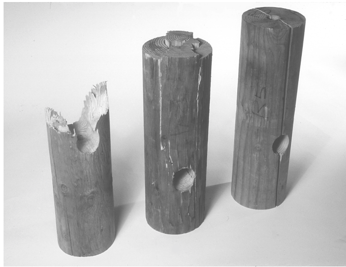
Figure 3. Predominant failure modes for dowel-nut connection
