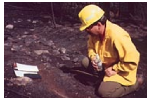
Geoff Cerrelli, NRCS civil engineer, tests the hydrophobicity of soil affected by fire.
