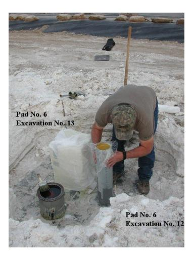
Appendix A9 – Field Sampling, Pad No. 6, Excavation 13 (Block Sample)
