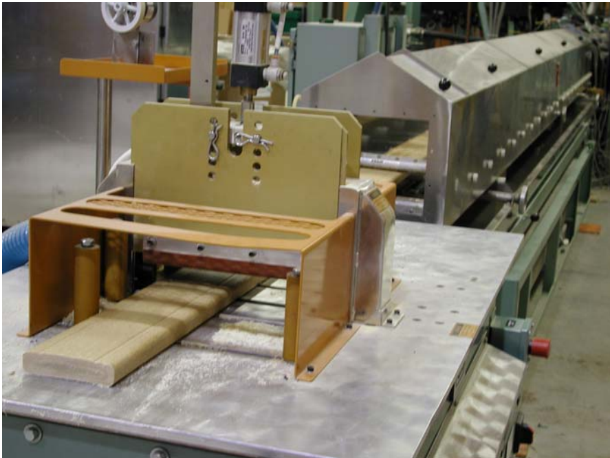
Figure 15: Wood-plastic composite exiting cut-off saw at end of profiling line.
