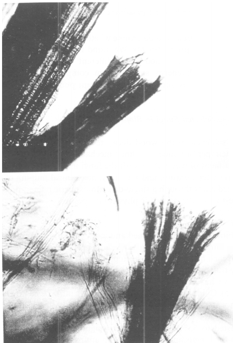
Fig. 4. Simons staining of control ( top ) and biopulp ( bottom ). Pulps from untreated control wood chips and Ceriporiopsis subvermispora - treated chips (4-week incubation) were passed through the refiner only once (Canadian Standard Freeness of pulps at about 700 ml) and then stained [80]
