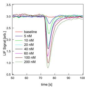
Data from integrated microfluidic device for monitoring water-borne nerve agents with 1 ppb limit of detection.
