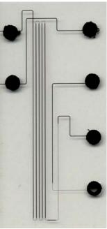
Microfluidic device for two-dimensional liquid phase separations of BW and CW agents. The microchip is 2"x 1" and the narrow channels are 75  $\mu$ m wide and 10  $\mu$ m deep. The microchannels and fluid reservoirs are filled with black ink for contrast.
