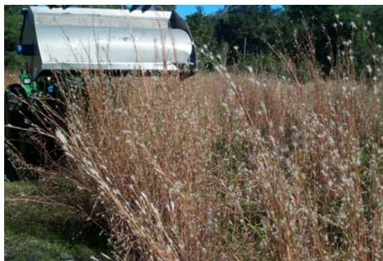
Harvesting Ft. Cooper Germplasm with a Woodward Flail-Vac seed stripper
