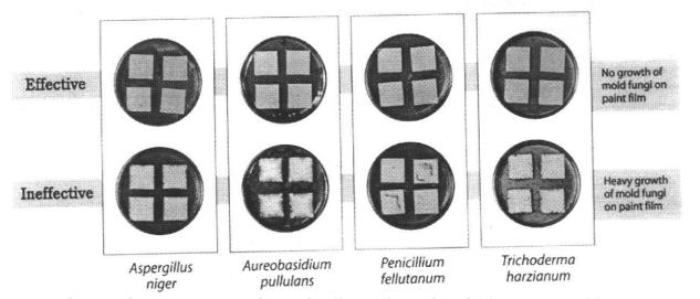
**Figure 2.**—The agar plate toxicity test evaluates the efficacy of paint biocides for resistance of four common mold fungi. Note the zone of inhibition that the effective biocide shows for Aureobasidium pullulans.
