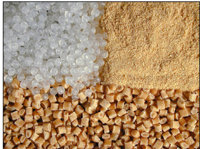
Clockwise from top left: virgin polyethylene pellets, wood flour, and wood-plastic composite pellets.
