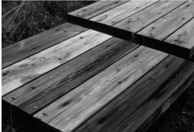
These experimental deck units demonstrate the beneficial effect of in-place preservative treatments.
