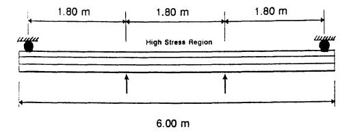
Fig 2: Beam test configuration
