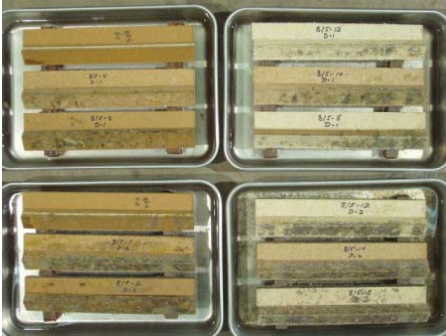
Fig. 3 evaluating potential for mould growth when woodfibre-rich (left) MDF is compared to CFF-rich MDF (right) after being exposed in a covered container and suspended above liquid water, but not in direct contact with that water [5].
