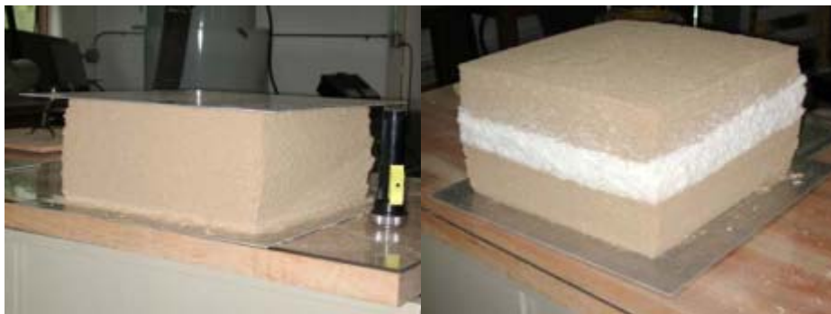
Fig. 2 examples of two pre-pressed MDF mats prior to pressing showing a uniform distribution of aspen fibre (left) and a three-layer mat with aspen fibre on faces and CFF in core (right).
