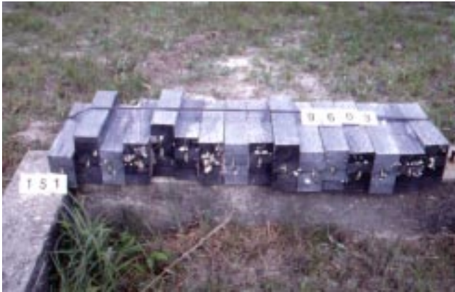
Figure 1—Units of treatment held together with metal banding and exposed in southern Mississippi in east–west direction longitudinally. Insertion holes were on the side toward the ground.
