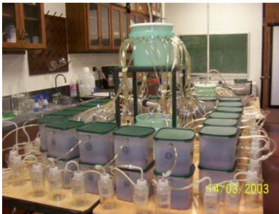
155 156 Figure 1. Photograph of the ammonia emission apparatus consisting of Tupperware® air emission chambers 157 and acid traps connected to a vacuum pump.
