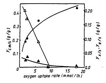
Yields of biomass (♠), xylitol (△), and ethanol (♠) on xylose as a function of the oxygen uptake rate of C. boidinii; dilution rate, 0.05 1/h.
