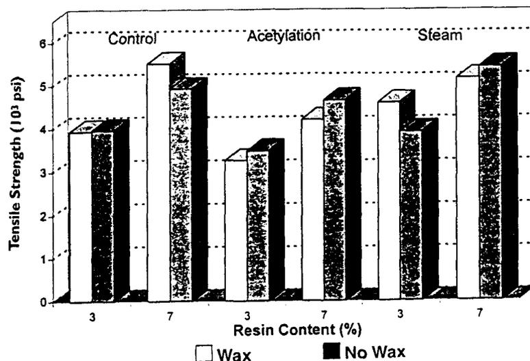
Figure 3. — Effects of treatment, resin content, and wax content on tensile strength parallel to the surface.
