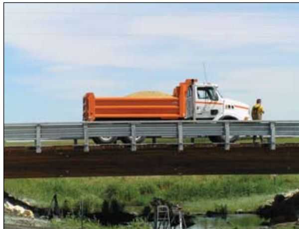
Evaluation of current load distribution criteria will be compared with results obtained from actual load testing.
