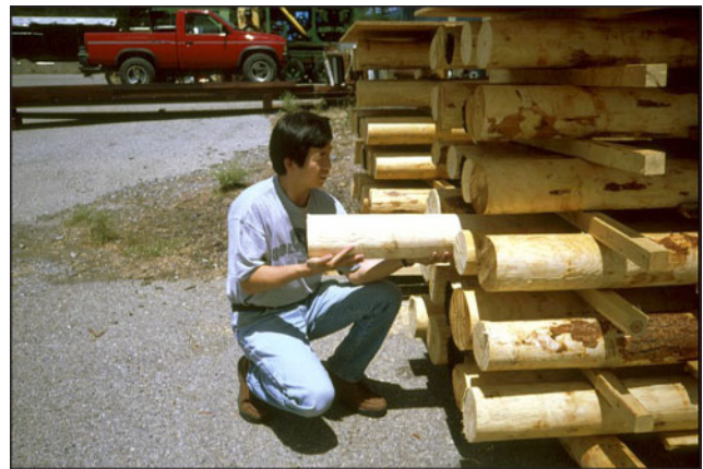
Figure 2—Moisture-content-monitored log section being removed for periodic weighing.
