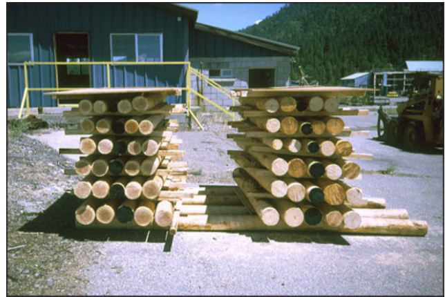
Figure 1—Air drying stacks of ponderosa pine and Douglas-fir logs in Hayfork, California. Black end-coated logs are moisture-content-monitored log sections.
