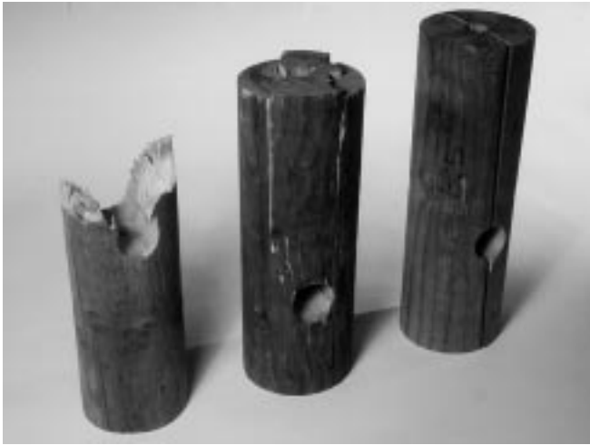
Figure 4—Shear, tension-perpendicular-to-grain, and tension-parallel-to-grain failures in test joints (left to right).
