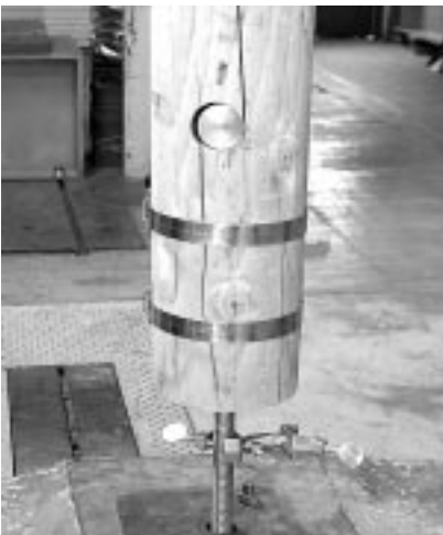
Figure 1—Dowel-nut connection detail.
