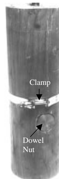
Figure 2—Steel-strap pipe clamp with threaded T-bar tightening device.
