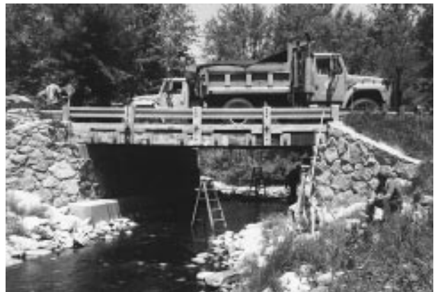
Figure 15—Transverse load positions used for load test 2. From top to bottom: load position 3, load position 6, load position 6 (side view) are shown.
