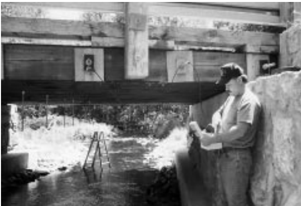
Figure 9—Obtaining a load cell reading with a portable strain indicator.
