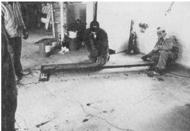
Figure 11—Measurement of bridge lamination MOE using the transverse vibration technique. Measurements were taken in the garage of the Centerville Water Department adjacent to the bridge site.
