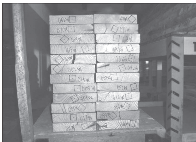
Figure 7—Tested lumber marked for cutting small clear specimens.
