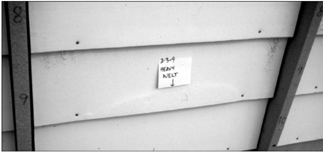
Figure 11—Example of edge welt on fence 2 (drip edges intact). Specimen was rated on August 25, 1999, as having a welt severity of 9.0 and a welt area of 21 in 2 (EWI = 21).
