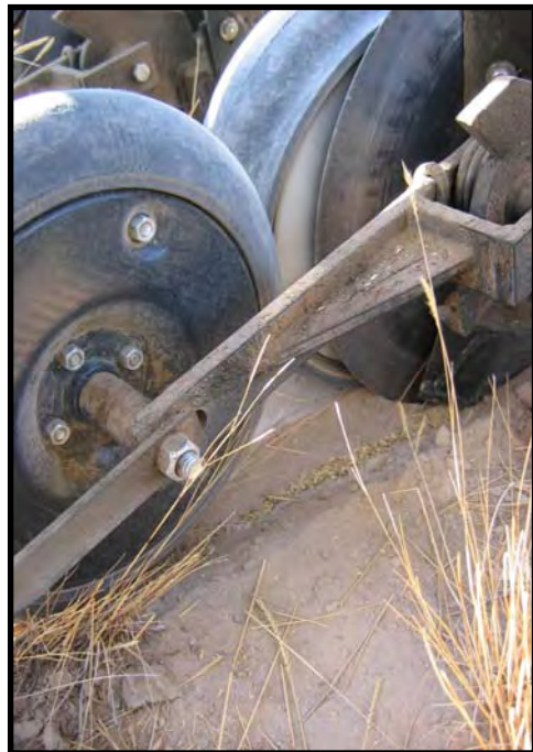
Photo 2.2. Wider disc opening in the soil for seed to drop into and press wheel adjustment to better cover seeds with soil behind disc openers.
