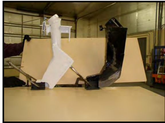
Photo 2.1. Re-designed seed drop tubes and boots (white boot) for a smoother flow of seed from the seed box to the soil.
