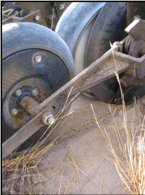
Wider disc opening in the soil for seed to drop into and press wheel adjustment to better cover seeds with soil behind disk openers.
