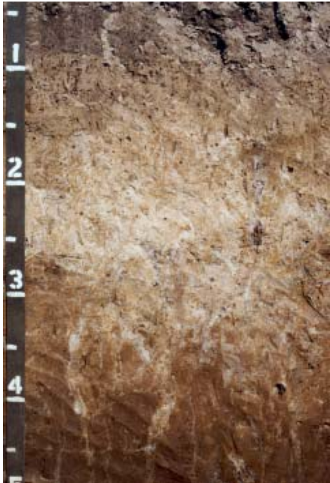
Figure 10.—Typical profile of Gumdale silt loam. The grayish colors between depths of 1.0 and 2.5 feet are caused by a perched water table. The brownish lower part is a dense fragipan.
