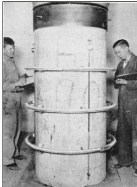
1.27. Concrete cylinder test for Hoover Dam, Arizona-Nevada
