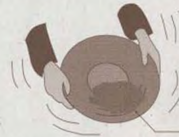
Figure 4. With the pan's riffles pointed away from you, alternate underwater dipping and swirling, until the lighter, finer material is washed away and the heavier material remains in the bottom of the pan.
