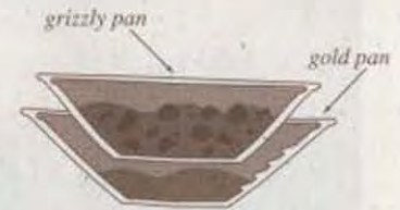
Figure 3b. Pan cross-section. After the rocks caught in the grizzly are examined for gold, they may be discarded.
