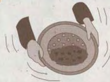
Figure 3a. A grizzly (a pan with holes in the bottom) is used to separate larger rocks from the finer material.
