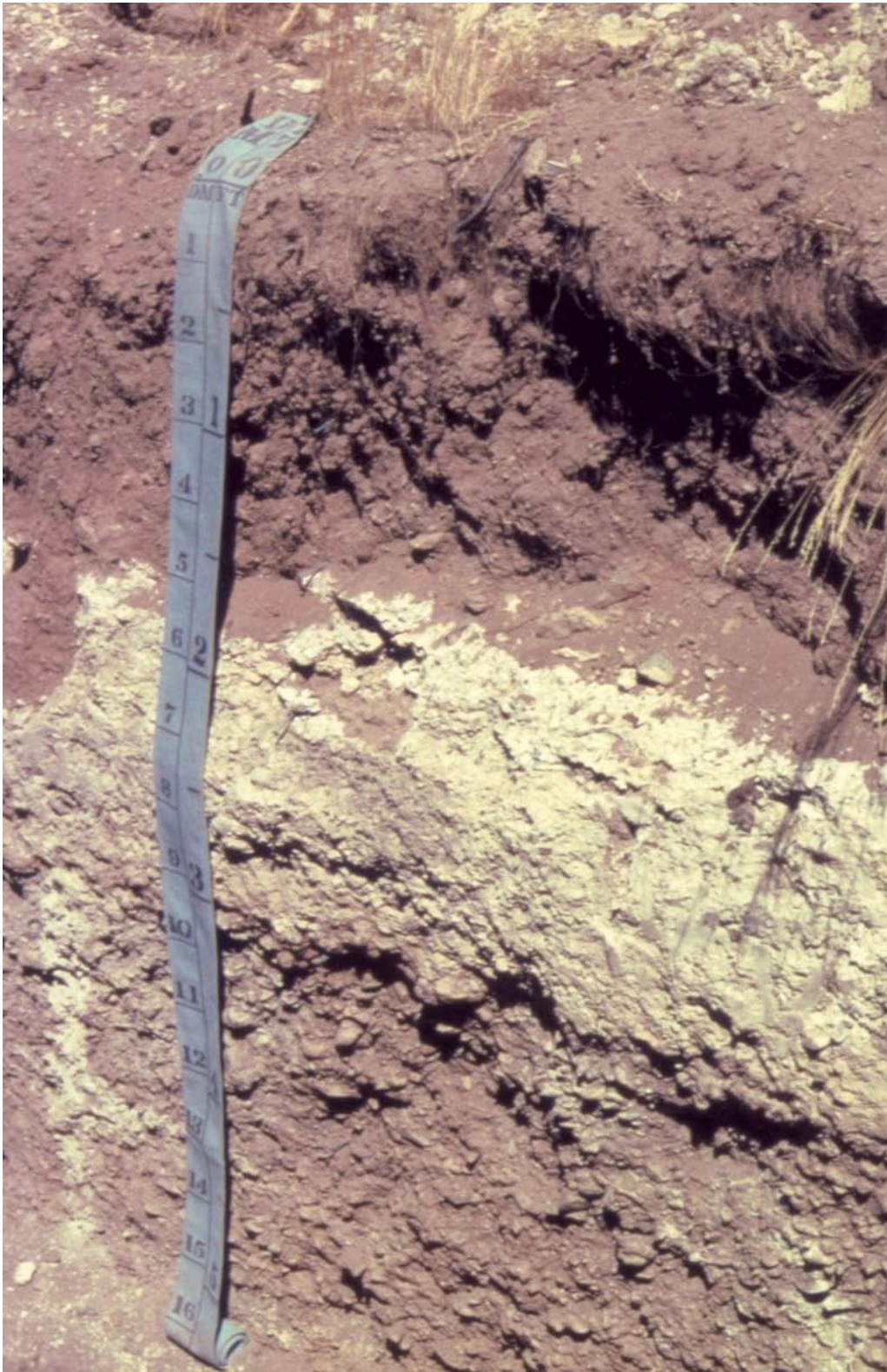
Figure 16.—Typical profile of a Stampede soil. A duripan is between depths of 23 and 33 inches. Very gravelly sandy loam derived from old alluvium is below the duripan.
