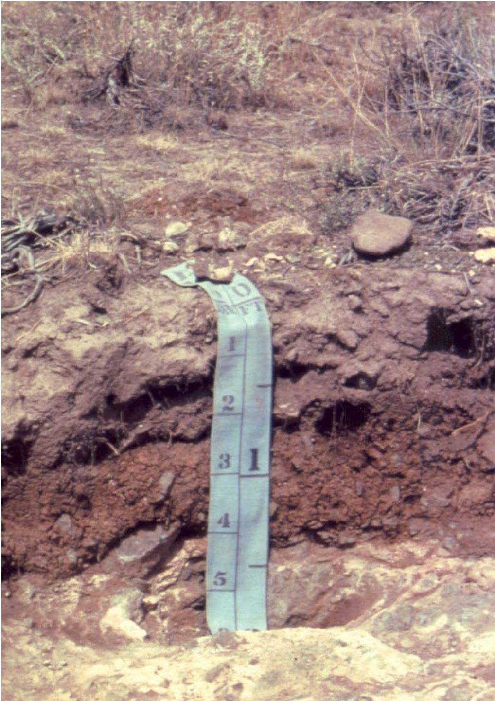
Figure 15.—Typical profile of a Ninemile soil. Basalt is at a depth of 16 inches. The upper 8 inches of the bedrock has discontinuous silica and carbonate pendants.
