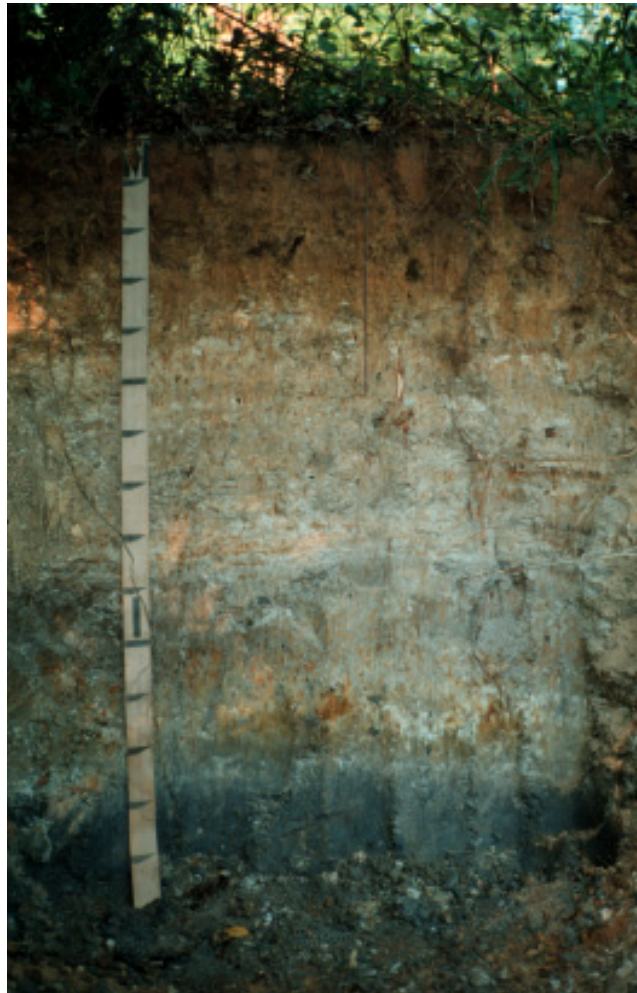
Figure 8. —Typical profile of Cartecay loam, frequently flooded, showing stratified layers deposited by flooding.
