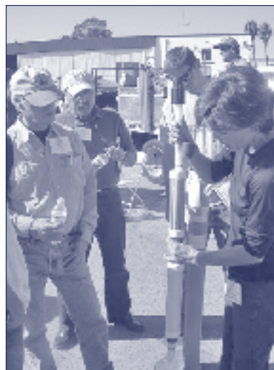
Kirstin Cooper from Solinst, Canada shows attendees a new three-channel multilevel monitoring system designed for direct push installation. Fluted bentonite cartridges seal the borehole between the sampling zones.
