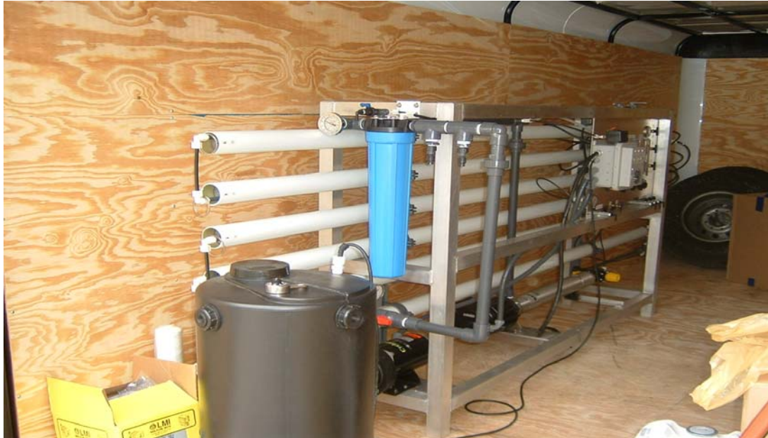
Figure 3-15. Second-Pass SWRO Photograph.
