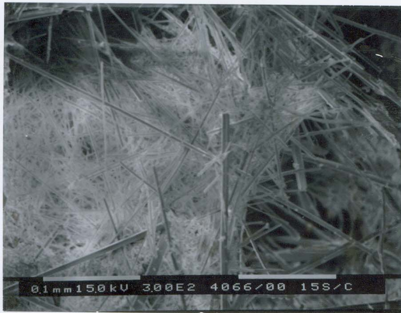
Figure 2. Electron Microscope Pictures of Calcium Sulfate Precipitate.
