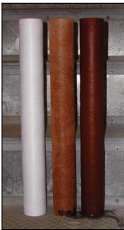
Figure 16 – Photograph Showing a New Cartridge Filter (Left) Next to Filters Fouled by Particulate Iron During Piloting at BPU.
