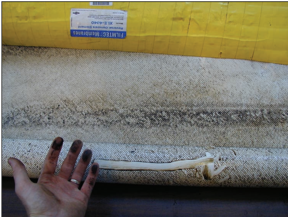
Figure 13 – Photograph Showing the Membrane Surface of the Membrane Element Fouled by Particulate Manganese During Run 1 at the DMWW.
