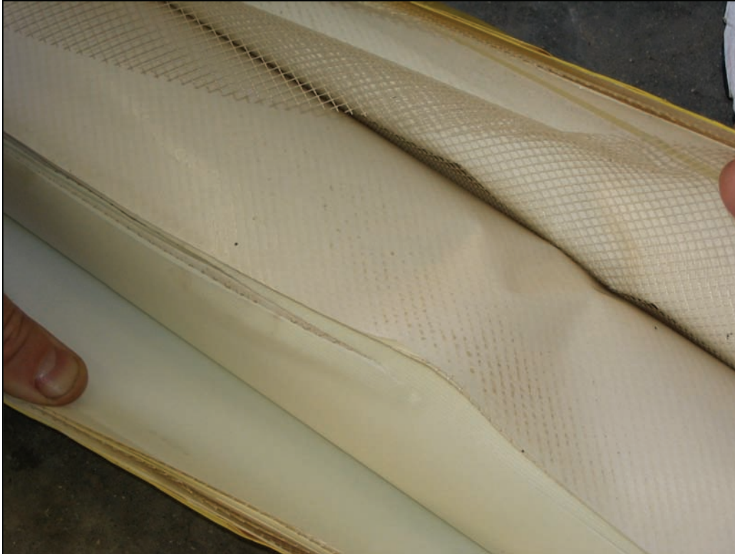
Figure 21 – Photograph Showing No Significant Fouling of the Membrane Following 75 Days of Operation at the LWC.
