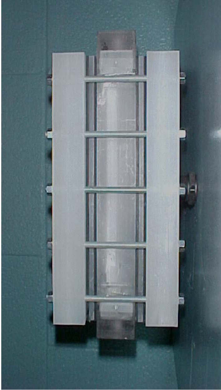
Figure 5. Rectangular crossflow test module with face boxes, plates, and assembly.
