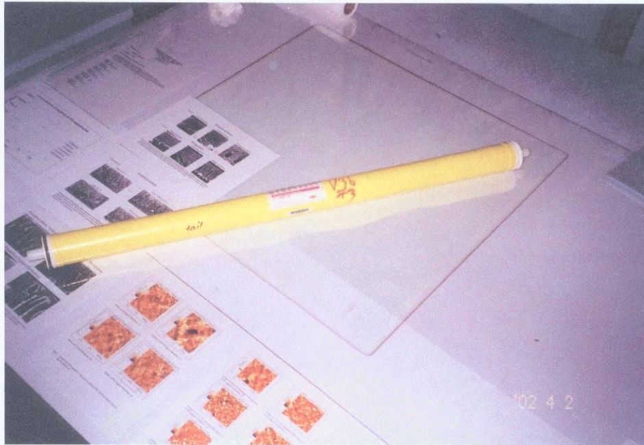
Figure 1 FilmTec NF-90-2540 A8425280. Tail element V3B#3 before autopsy. Morana, AZ. pilot test 10/10 – 03/02
