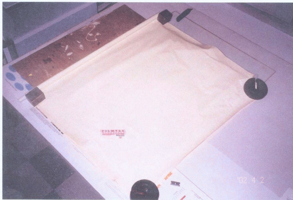
Figure 1 FilmTec NF-90-2540 A8425281. Lead element V1A#1 before autopsy Morana, AZ. pilot test 10/01 – 03/02
