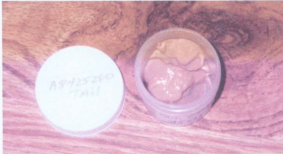
Figure 3 FilmTec NF-90-2540 A8425280. Tail element V3B#3 foulant collected. Morana, AZ. pilot test 10/01 – 03/02
