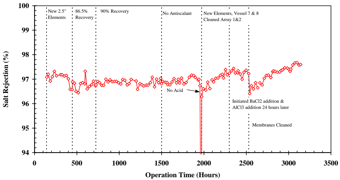
Figure 32. Salt rejection during reverse osmosis pilot testing
